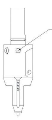
Pressure is reduced by turning in the clockwise direction. The **YELLOW** screw can be turned approx. 7mm to maximum reduction.
