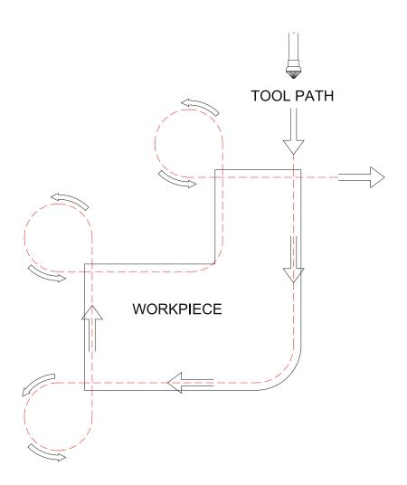
CNC Deburring Tool-Path on workpiece contour
