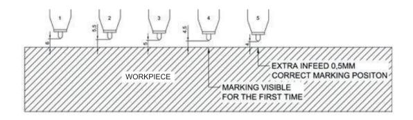
While approaching to the workpiece marking needle hit the first dot multiple times and makes the entrance of the first character deeper. After determining the correct marking position approaching towards the marking position should be as fast as possible to minimize this.
