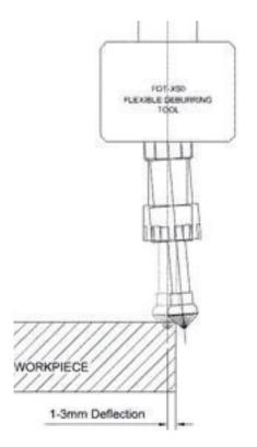
Cutting Direction: FDT deburring tools, the cutter rotation should be clockwise when viewed from above. Climb milling would therefore involve clockwise motion around the part being deburred.
