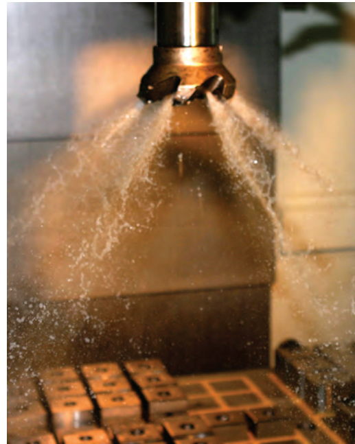
CoolBLAST arbor screw provides coolant path.
