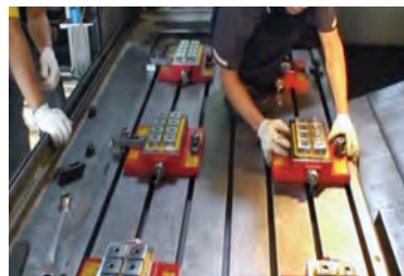
Position the chucks on the machine bed
