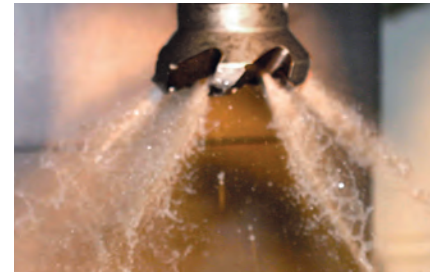
CoolBLAST arbor screw provides coolant path.
