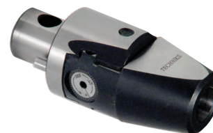
Use Micro Heads with Boring Bars
