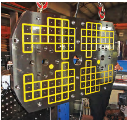
Load and install PIM magnet with bolts
